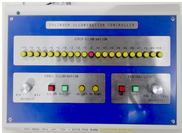
Figure 2: Lighting control panel for OBACHT. Each LED strip can be activated individually, and their collective intensity adjusted. The central light, comprising three white LEDs behind the semi-transparent mirror, can have its intensity adjusted independently.
