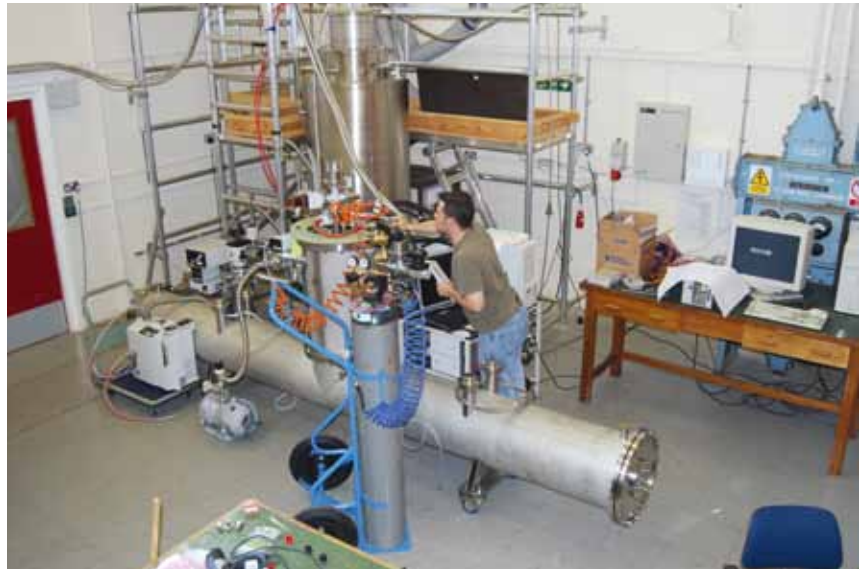
Figure 3.22 The 4-m prototype superconducting helical undulator under test at Rutherford Appleton Laboratory.
