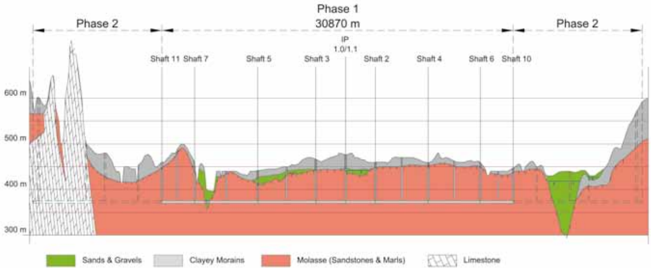
Figure 5.15 Tunnel geology of the CERN region.
