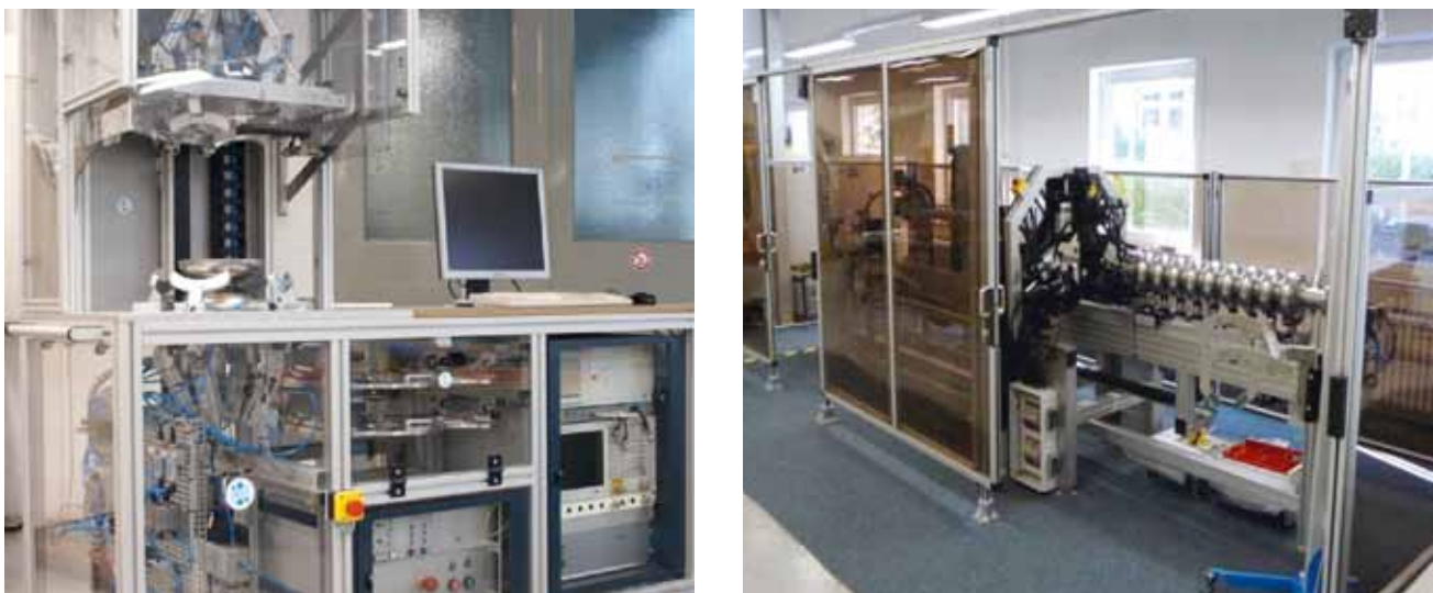
Figure 2.12 Left: tool for room temperature RF measurement of half cells. Right: tool for field flatness tuning of completed cavities.
