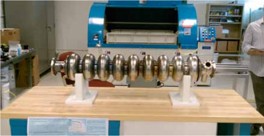
Figure 2.9 The Fermilab tumbling process facility.
