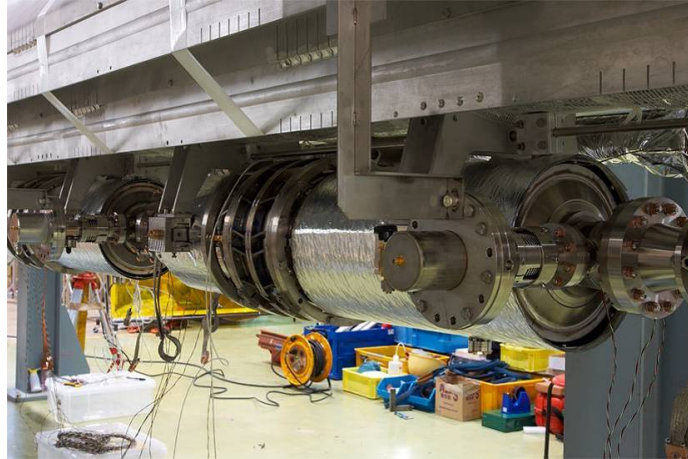
Figure 30 One of the Blade Tuner cavity suspended on the cold mass of the cryomodule
