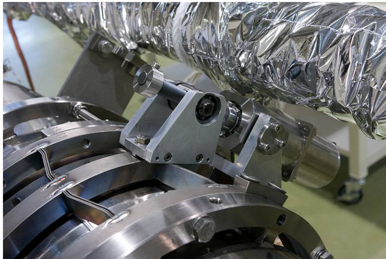
Figure 29 A closer view of the motor drive unit installed for the Blade Tuner
