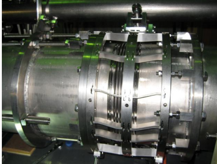
Figure 17 T the new ILC Blade Tuner installed on the Z86 cavity. The adaptation elements are also visible.
