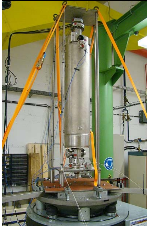
Figure 3 Vibration test stand at the institute BFSV that carried out acceleration studies of the transport frame with the cavity under well-defined conditions.
